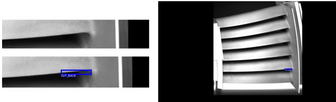
Figure 42 – Single-defect model – Background misclassified as defect
