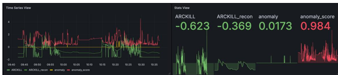
Figure 72 – Anomaly detection output example in two separate visualisations. On the left, the signal is deemed as anomalous and, on the right, the specific anomalous pattern is accompanied by a numerical indication of the anomaly score
