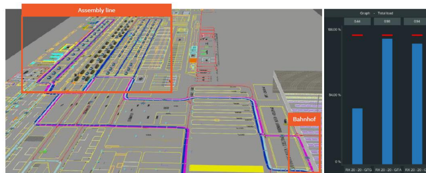
Figure 7 - Asset occupation of the actual GT Process through simulation.
