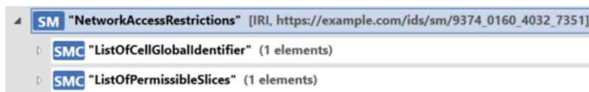
Figure 80: NetworkAccessRestrictions submodel of a 5G UE Digital Twin or AAS.
