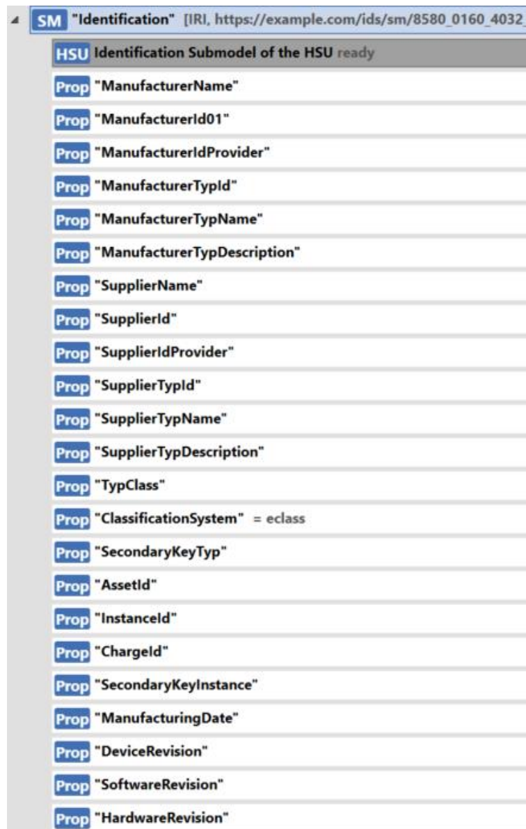
Figure 74: Identification submodel of a 5G UE Digital Twin or AAS.
